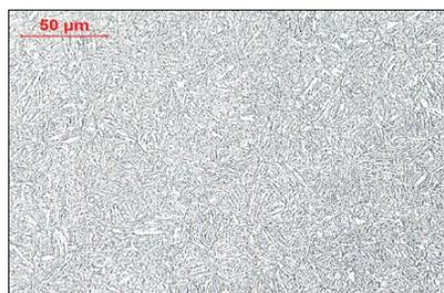
**Delivery condition:** EAF, VAD, 3D-forged, EFS treated (extra fine microstructure)
